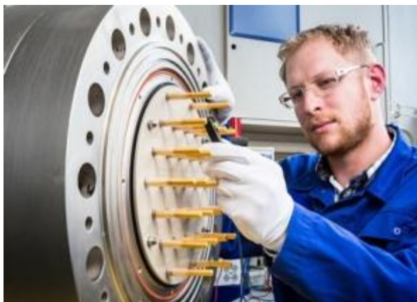
Final quality checks of a glass-to-metal sealed SCHOTT Eternaloc® electrical penetration assembly.
